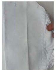
The final wash was adjusted from a cold short wash to a medium 60c wash, with the addition of normal washing powder.
